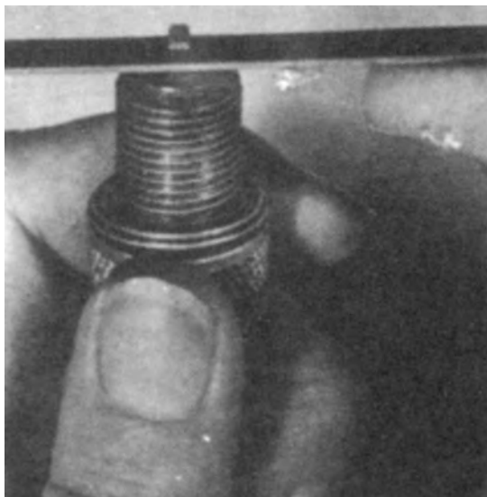
Fig. 11.65 Filing the electrodes
