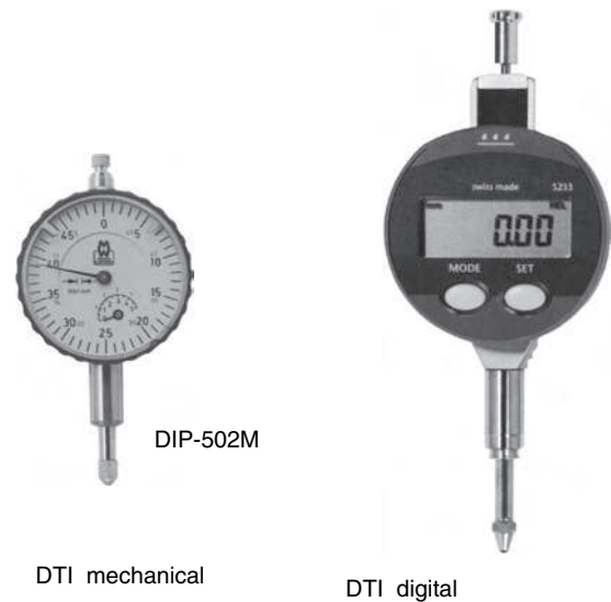
Fig. 13.12 Dial Test Indicators DTIs
