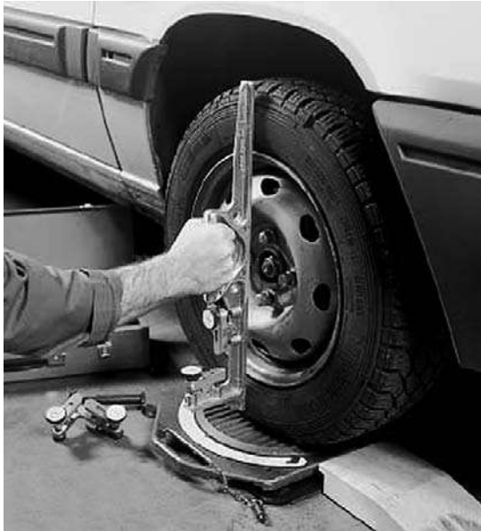
Fig. 22.41 Camber gauge in position (Sealey garage equipment)
