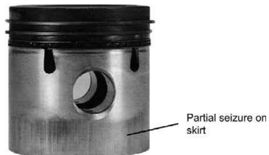
Fig. 3.23 Damage at piston skirt
