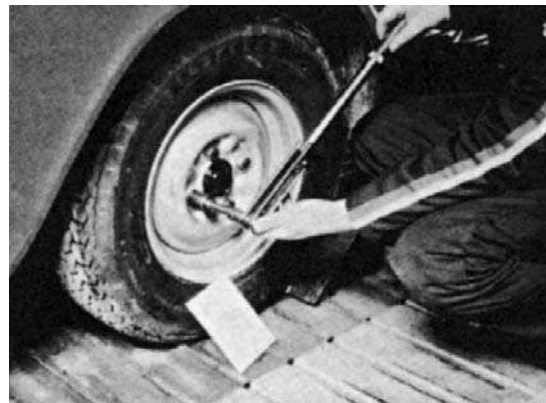
Fig. 22.30 Using a torque wrench for the final tightening
