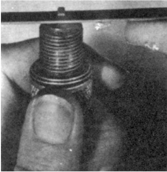
Fig. 27.53 Filing the electrodes
