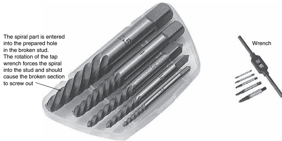
Fig. 30.10 Screw extractors
