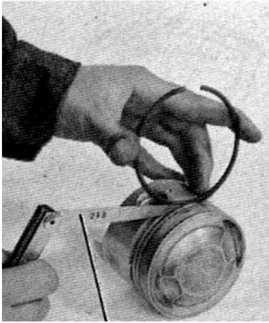
Fig. 3.24 Piston ring side clearance in the piston
