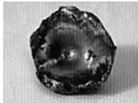
Valve head broken off
