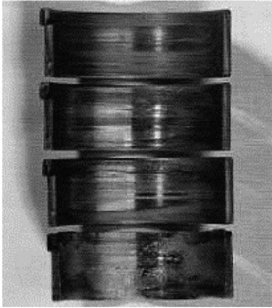
Fig. 17.7 Big-end bearing failures
