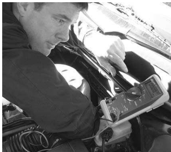
Figure 9.56 Circuit voltage testing
