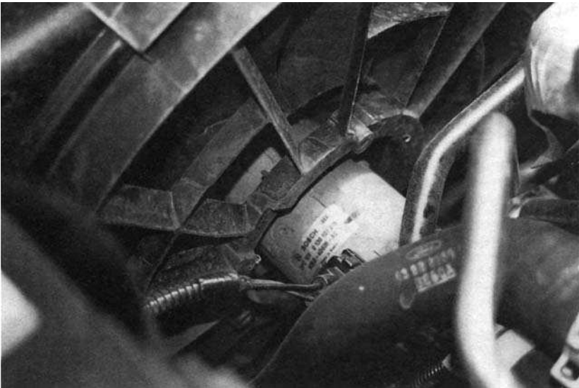
Figure 9.23 Cooling fan motor
