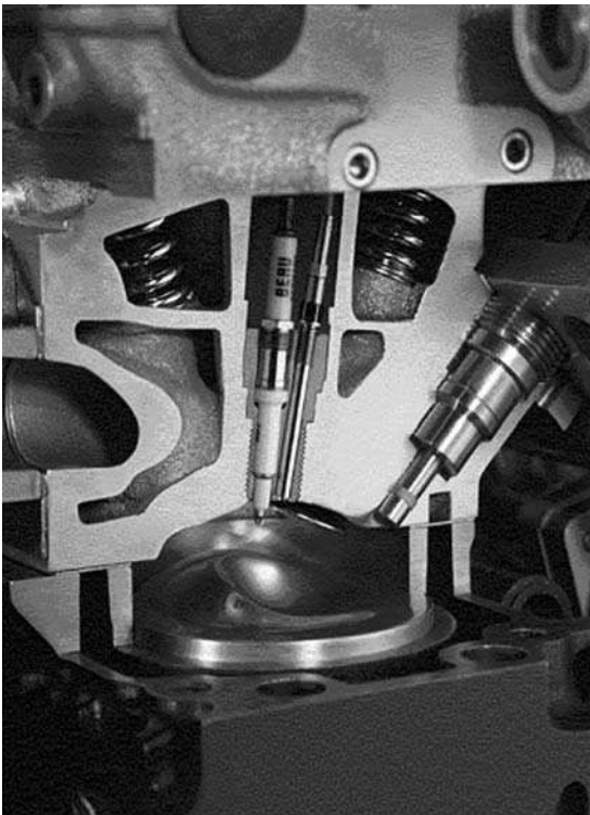
Figure 5.28 Cylinder pressure sensor mounted in the engine
