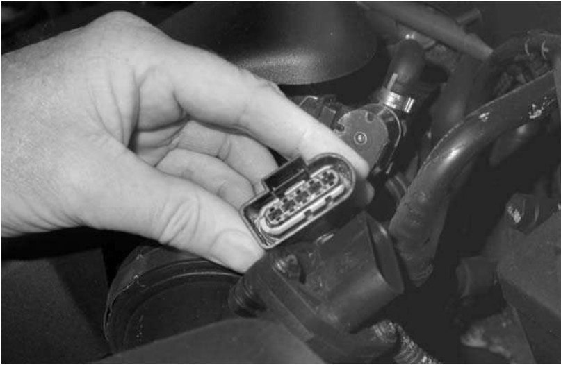
Figure 7.43 Air flow meter under test
